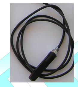
One *optic head* for the check of holes and dropped stitches in the produced fabric. The optic head is placed directly onto the produced fabric to see holes and dropped stitches.
