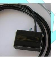
Otherwise from the models AG and AGF preceding, the optic needle scanner is connected directly to the main unit.
