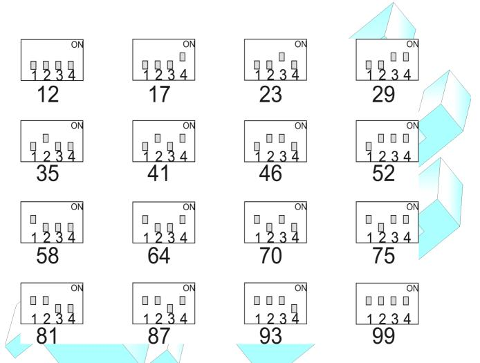
It is up to the system integrator to set the dip-switch at the proper value for each textile machine.
