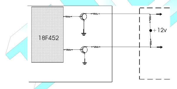
Maximum current is 100mA, maximum voltage is 16V.
